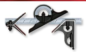
A complete substitute for a whole set of common solid try squares, a 45 degree mitre, a depth gauge, a height gauge, a marking or scribing gauge, a level, a plumb and by withdrawing the blade, it can also be used as a precision rule.
